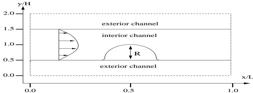
FIGURE 1. A schematic of the computational domain (bounded by the dashed lines) used by the immersed boundary method, for computing the left-to-right pressure-driven viscous flow through a channel of length  $L$  and height  $H$  (solid lines). In §4, we study Poiseuille flow where  $R = 0$ , however in §6, we assume  $R > 0$ .
