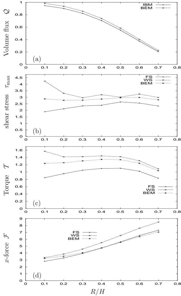
FIGURE 5. Comparisons of four quantities:  $x$ -force, torque, maximum shear stress and volume flux using the IMBM and BEM, in non-dimensional units. For (b-d) the IMBM has two results obtained by using the fluid stresses (FS) and the wall stress (WS). The calculations were performed on a  $512 \times 128$  grid with  $H/L = 1/8$ . The fluid stress was evaluated one grid-point inwardly normal from the wall at  $\mathbf{X} - \mathbf{n}h$ .
