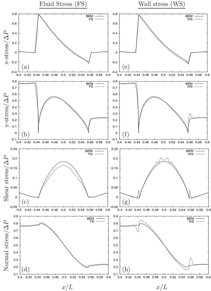
FIGURE 4. Comparison of dimensionless fluid stresses on the lower channel wall for  $R/H = 1/2$  and  $H/L = 1/8$  computed using the immersed boundary fluid stress (FS) and the immersed boundary wall stress (WS). The solid line in each figure is the BEM solution. For the IMBM, a  $512 \times 128$  grid with one-way flow was used, with the FS evaluated one grid-point inwardly normal from the wall at  $\mathbf{X} - \mathbf{n}h$ .
