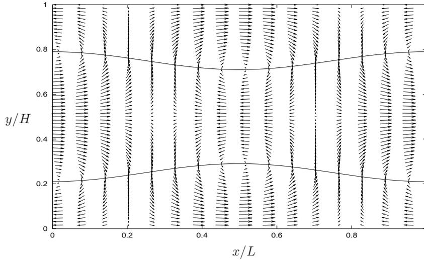
FIGURE 6. A velocity vector field, in the laboratory frame of reference, of a peristaltic pumping flow generated using the IMBM at  $t = 7.5$ s, after two complete cycles. The computational domain is periodic in both orthogonal directions.
