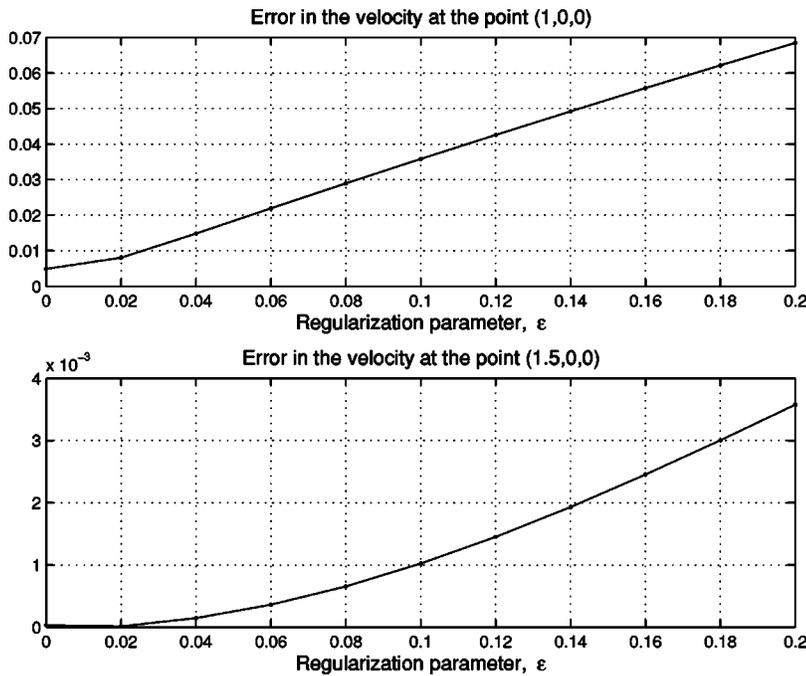
FIG. 5. Numerical computation of the velocity at two different points in the fluid for various values of  $\epsilon$ . The discretization was fixed with a  $60 \times 60$  grid on each of the six patches. The top graph shows the velocity error at a point on the surface of the sphere; the bottom graph shows the velocity error at a point far from the surface.
