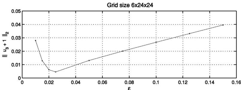
FIG. 2.  $L_2$  norm of the error in the third component of velocity on the sphere as a function of the regularization parameter  $\epsilon$ . The surface of the sphere was discretized using a six-patch  $24 \times 24$  fixed grid.
